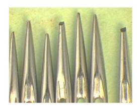
Broken needle points because the needle has touched some machine parts.
